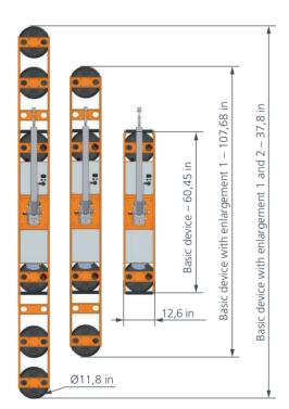
Basic device with enlargement 1 and lateral coupling flanges
